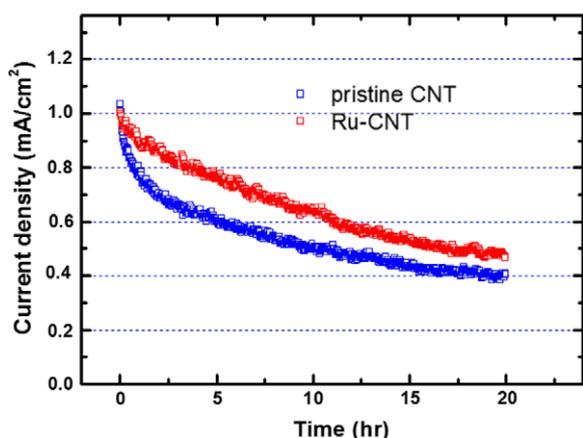
Fig. 6 – Lifetime comparison between pristine CNTs and Ru-CNTs. Measurements are performed at 1 mA/cm<sup>2</sup> under dc voltage for 20 h.
