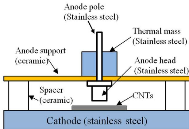
Fig. 1 – Schematic of field emission measurement setup.
