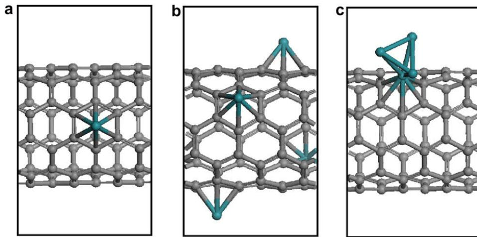
**Fig. 8 – The unit cell of a (5,5) CNT with the Ru attachment types. (a) One and (b) four Ru atoms are attached. (c) A Ru<sub>4</sub> cluster is adsorbed.**
