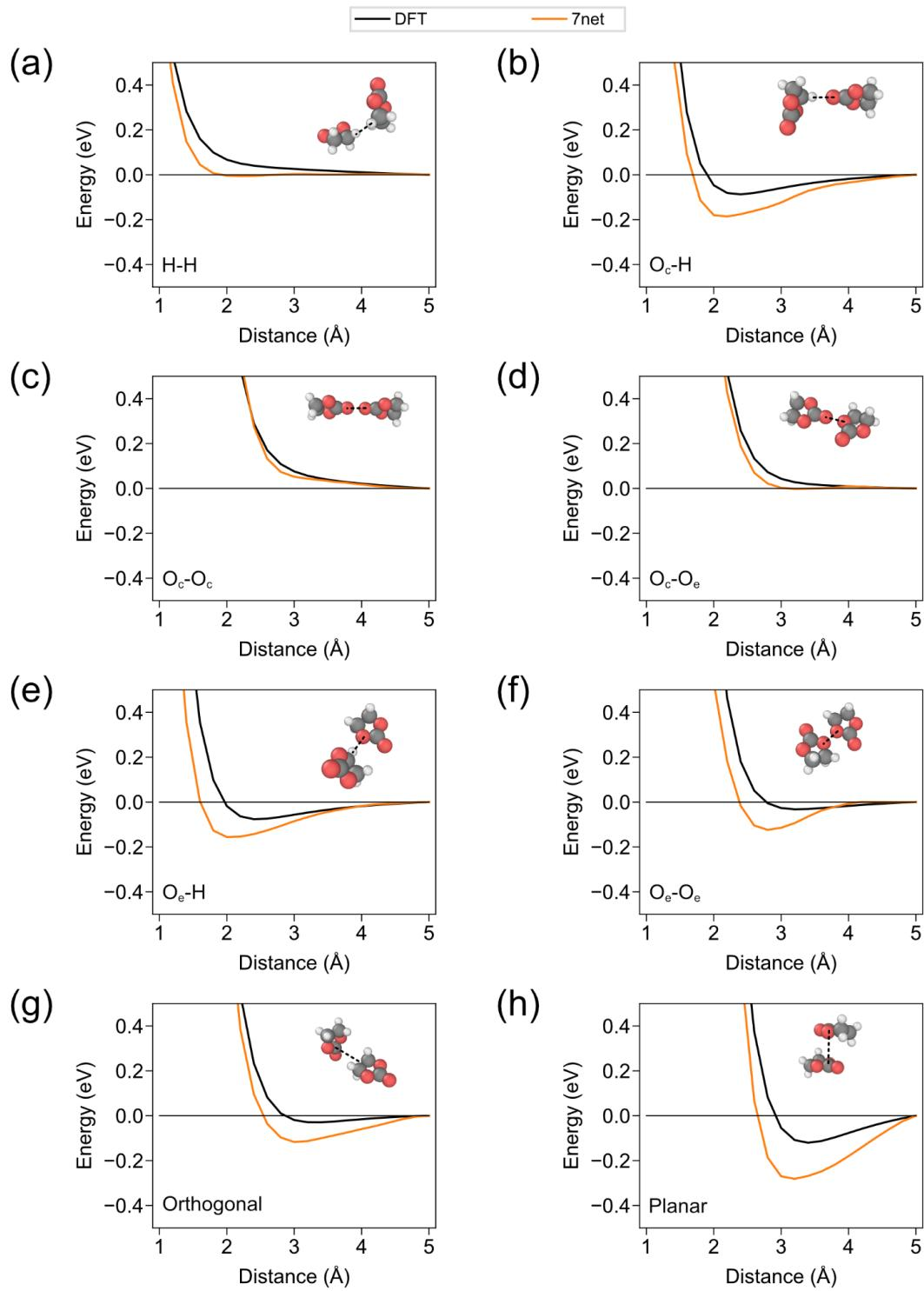
**Figure S3.** Potential energy curve of EC dimer obtained from SevenNet compared to DFT values according to the distance of (a) H-H, (b)  $\text{O}_c\text{-H}$ , (c)  $\text{O}_c\text{-O}_c$ , (d)  $\text{O}_c\text{-O}_e$ , (e)  $\text{O}_e\text{-H}$ , (f)  $\text{O}_e\text{-O}_e$ , (g) orthogonal orientation of dimer ( $\text{C}_c$  and positional average of 4 hydrogen), and (h) planar orientation of dimer ( $\text{C}_c$  and  $\text{C}_{\text{e}}$ ).
