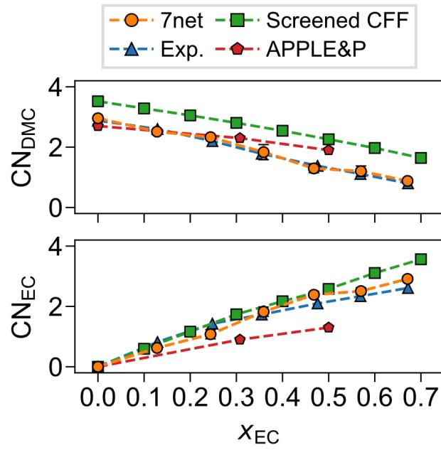
**Figure S10.** Average CNs of Li contributed by EC and DMC solvents in EC/DMC (1 mol/kg LiPF<sub>6</sub>) electrolyte at 298 K compared with experimental values<sup>6</sup> and results obtained from other force fields (Classical force fields with screened Coulomb interaction<sup>7</sup> and APPLE&P<sup>8</sup>).
