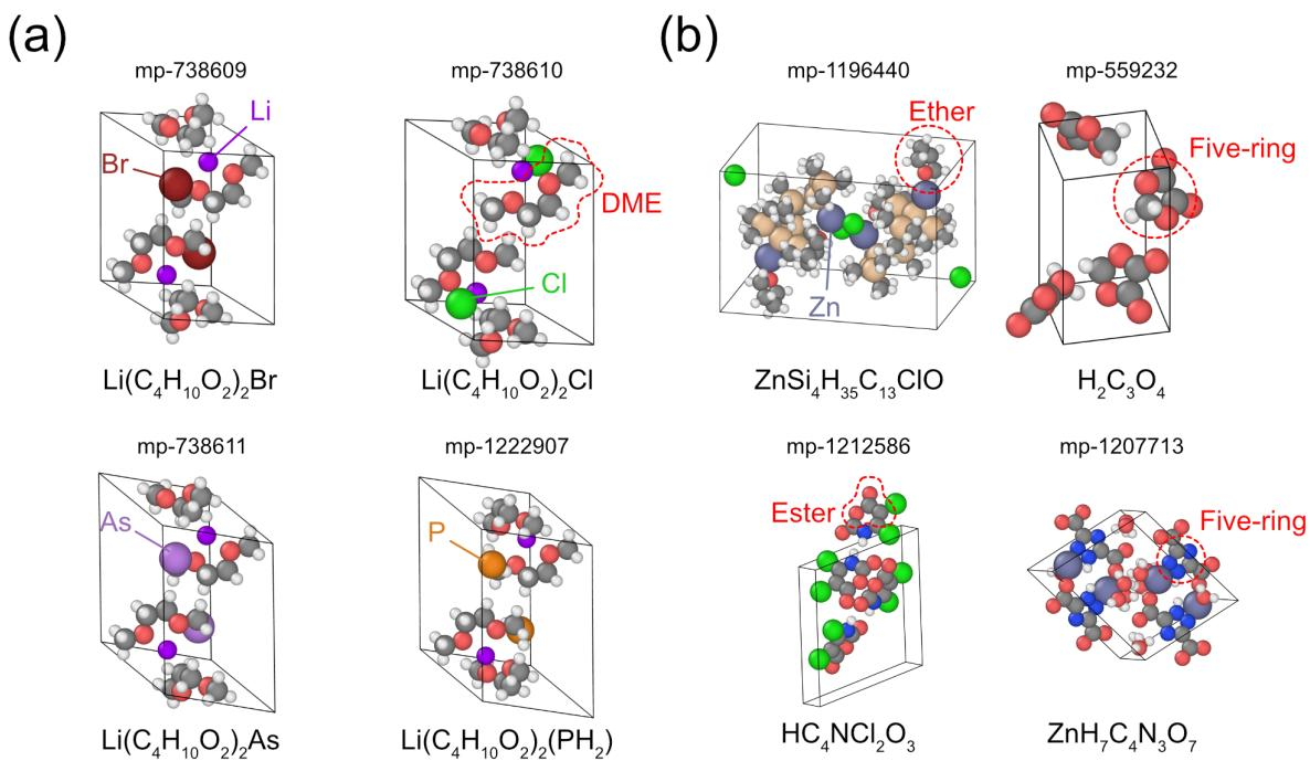
**Figure S12.** Similar or identical molecules with our solvent set in the training data. (a) All four structures in the training set that include DME molecules. (b) Representative similar molecules identified in the training set, featuring ether or ester groups, or containing five-membered ring structures.
