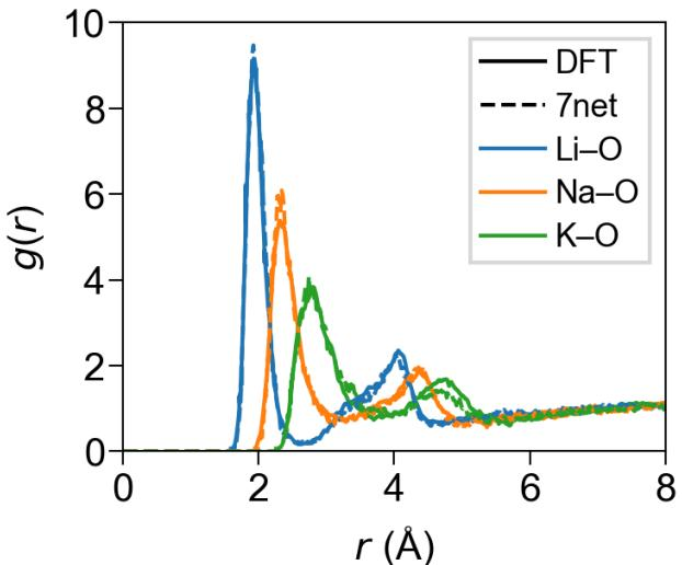
**Figure S7.** Radial distribution functions of Li, Na, and K cations between oxygens when solvated in EC molecules. Blue, orange, and green lines represent radial distribution functions from Li, Na, and K, respectively. The solid and dashed lines represent the results obtained from DFT calculations<sup>4</sup> and SevenNet, respectively.
