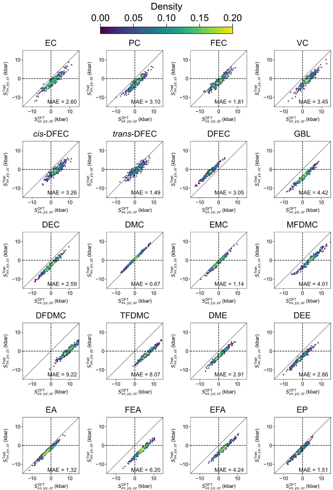
**Figure S17.** Normal stress parity plots for pure solvents calculated with SevenNet-FT.
