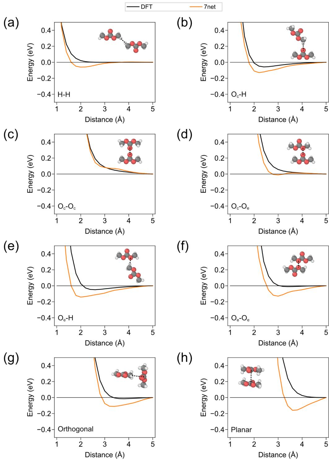
**Figure S4.** Potential energy curve of DMC dimer obtained from SevenNet compared to DFT values according to the distance of (a) H-H, (b) O<sub>c</sub>-H, (c) O<sub>c</sub>-O<sub>c</sub>, (d) O<sub>c</sub>-O<sub>e</sub>, (e) O<sub>e</sub>-H, (f) O<sub>e</sub>-O<sub>e</sub>, (g) orthogonal orientation of dimer (C<sub>c</sub> and positional average of 4 hydrogen), and (h) planar orientation of dimer (C<sub>c</sub> and C<sub>e</sub>).
