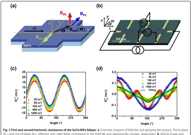
$(B_{FL})$  and out-of-plane  $(B_{DL})$  effective spin-orbit fields correspond to the field-like and damping-like torques, respectively. **b** Optical image and measurement geometry of the GeTe/NiFe hybrid device. **c**, **d** Transverse resistances of the first (**c**) and second-harmonic measurements (**d**). In **d**, the experimental data agree with the solid lines, which are the fits obtained from Eq. (2) ( $I_{AC} = 3$  mA).
