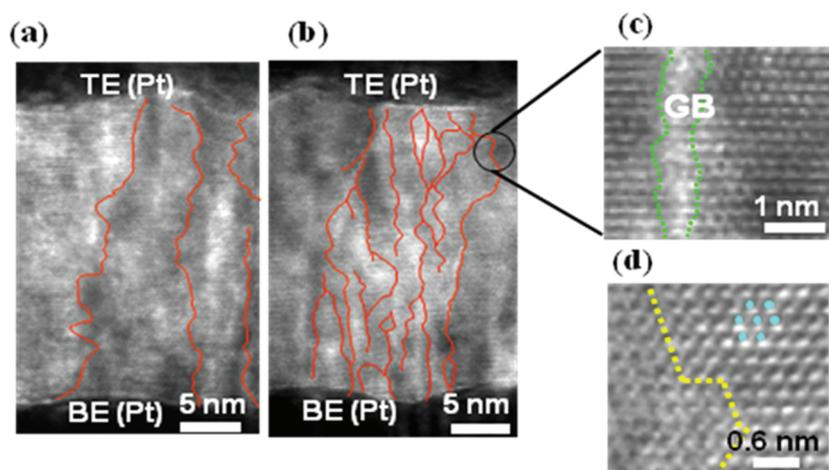
**Figure 3.** HR-TEM analyses of structural changes in memory switching NiO. Cross-sectional HR-TEM images of 5% NiO films (a) before and (b) after applying  $V_{\text{set}}$ . (c) An enlarged HR-TEM image near a grain boundary in Figure 3b. (d) Atomic image obtained near edge between grain and grain boundary in Figure 3c.
