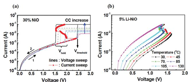
**Figure 4.** Threshold switching characteristics. a) Data obtained from double voltage sweep measurements ( $0\text{ V} \rightarrow 3\text{ V} \rightarrow 0\text{ V}$ ) under various compliance currents and single current sweep measurement ( $0.1\text{ mA} \rightarrow 100\text{ mA}$ ) for 30% NiO. (b) Data obtained from single current sweep measurement ( $0.1\text{ mA} \rightarrow 30\text{ mA}$ ) for 5% Li-NiO sample at temperatures from 30 to 130 °C.
